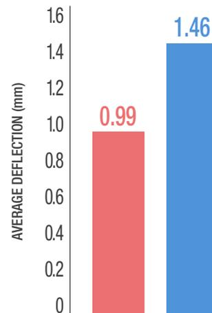
Comparative deflection (mm) of needle after penetration through a 10mm block of silicone<sup>2</sup>
