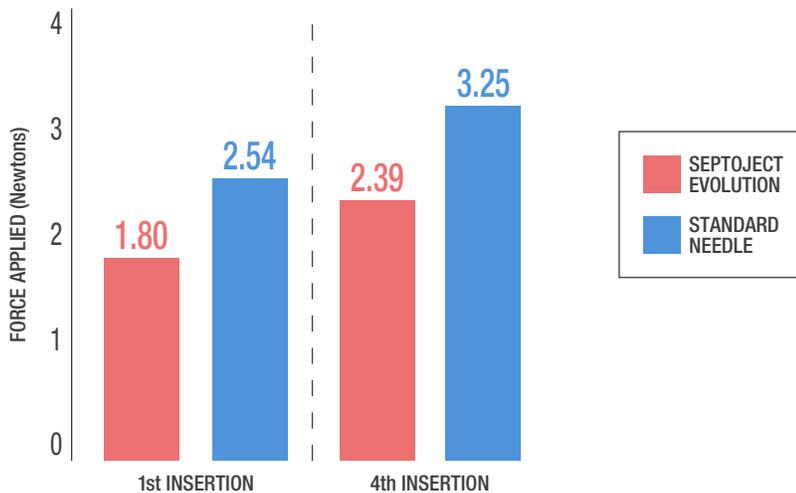
Force required (Newtons) for a 10mm penetration of a silicone block<sup>1</sup>
